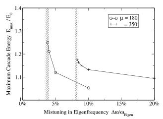
Fig. 13 Maximum cascade energy over mistuning amount.
