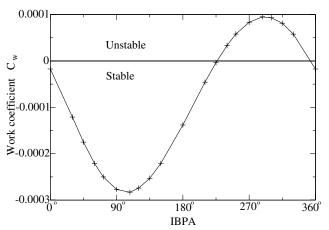
Fig.  $1\,$  Work coefficient of the tuned cascade vs interblade phase angle, uncoupled.
