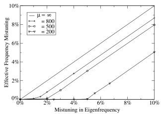
Fig. 9 Effective mistuning vs nominal mistuning for mass ratios 200 and 500.
