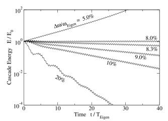
Fig. 11 Total energy of the cascade vs time for mass ratio 180.
