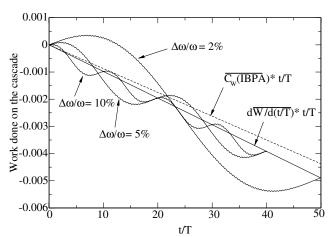
Fig. 2 Computed work on cascade with different amounts of mistuning by uncoupled method.
