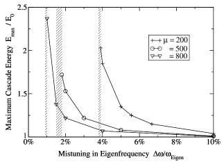
Fig. 8 Maximum cascade energy over mistuning amount.
